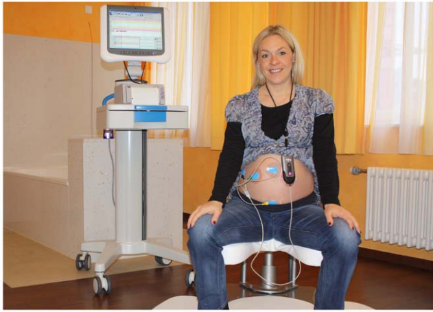
Figure 1. Fetal ECG monitoring device (MONICA AN24). Copyright and courtesy of Monica healthcare limited. Portable trans-abdominal fetal ECG monitoring device with 5 electrodes attached to the maternal abdomen. doi:10.1371/journal.pone.0028129.g001
